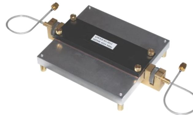
TE<sub>01δ</sub> cavities, typically 1 – 10 GHz
