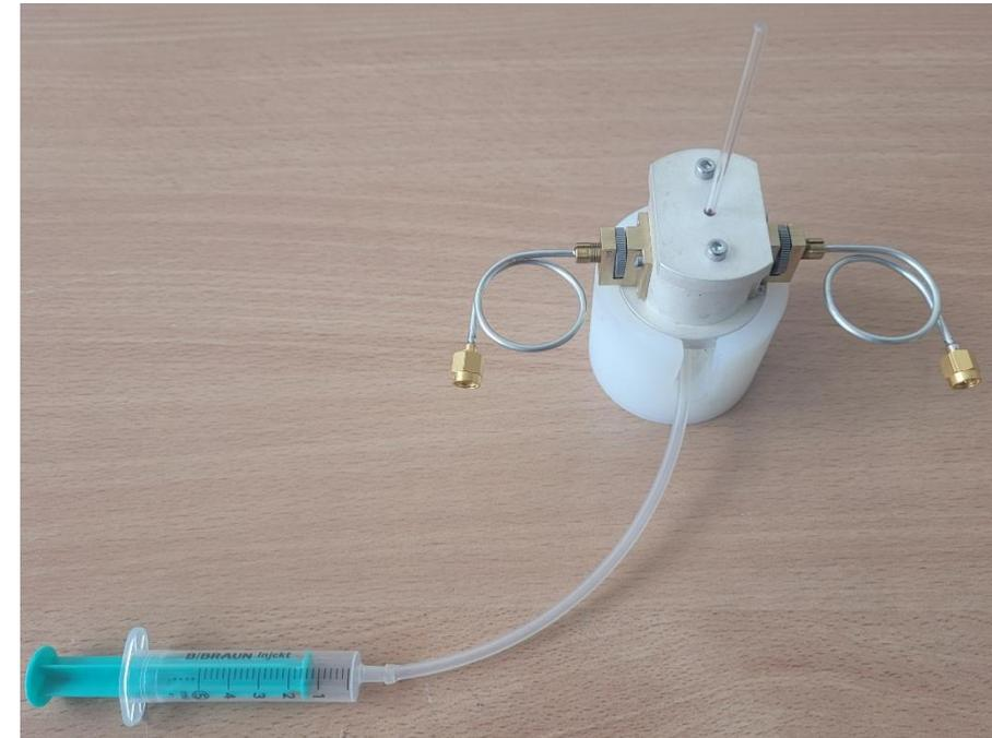
**24-GHz Cavity resonator**
