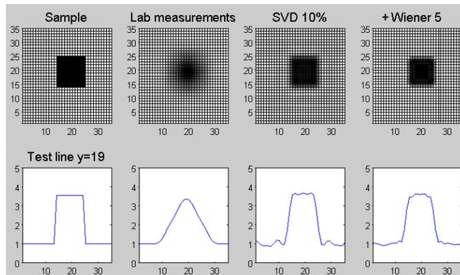
Fig. 6. MATLAB displays demonstrating the application of the SDI method to the permittivity image from the laboratory scanner with 10 GHz SPDR.
