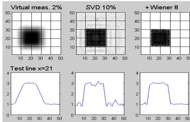
Fig. 5. Virtual experiment as in Fig. 4 but with random noise increased to 2%.
