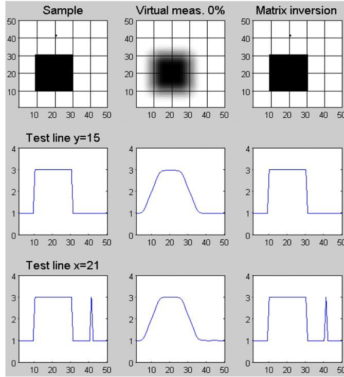
Fig. 2. Virtual measurement (with no added noise) of 20 mm x 20 mm sample and 1 mm dot on 50 mm x 50 mm background - and image reconstruction in MATLAB environment.
