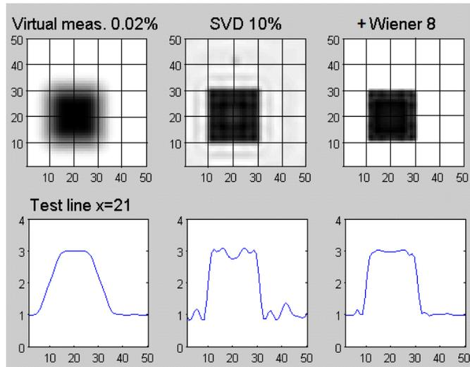
Fig. 4. Virtual experiment as in Fig. 3 but applying matrix regularisation with 10% eigenvalues retained.
