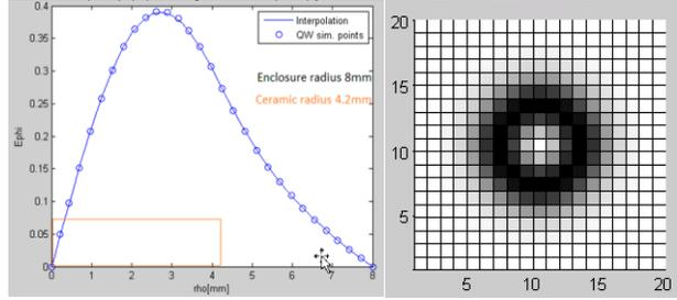
Fig. 1. E-field pattern of 10 GHz SPDR: left - radial distribution of azimuthal E-field simulated with BOR FDTD [7]; right - SPDR template (squared E-field extrapolated in MATLAB onto 1 mm mesh over the SPDR head).
