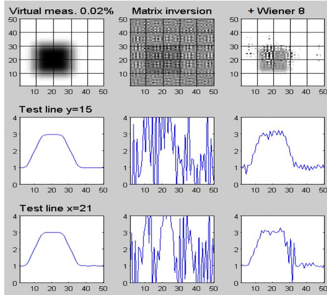
Fig. 3. Virtual measurement as in Fig. 2 but with random 0.02% noise added -and image reconstruction in MATLAB environment.
