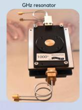
RF-nanoscale broadband techniques New nanoscale broadband GHz techniques to measure local SEI electrochemical activity and impedance changes, at large electrical bandwidth (milli Hz to Giga Hz), high temporal (<1 nano-second) and lateral (1-20 nano-meter) resolutions
