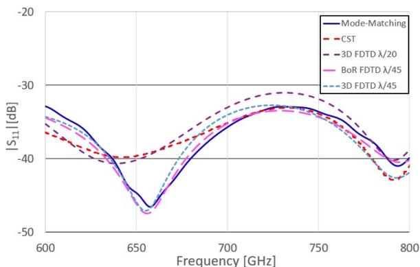
Fig. 5. Return loss calculated using different methods: Mode-Matching, 3D FDTD (CST[24] and in-house test code) and BoR FDTD [21] with conformal mesh generated by NanoBat Modeller [23].
