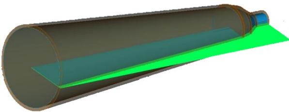
Fig. 2. 3D view of the considered multiflare antenna in NanoBat FreeCAD Modeller [23], which automatically generates 2D BoR mesh.
