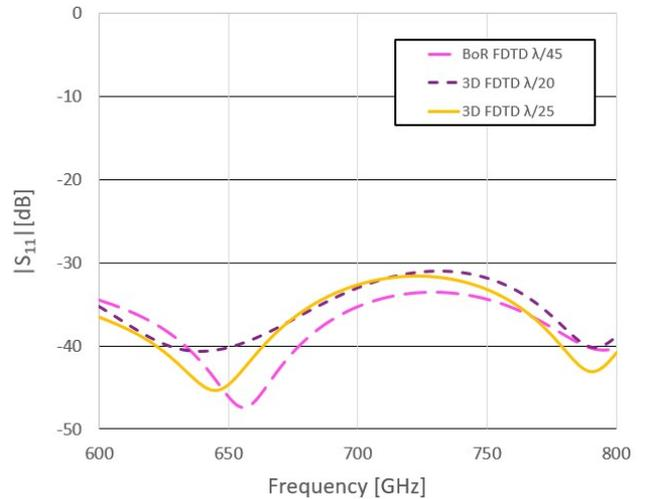
Fig. 4. Return loss calculated by 3D FDTD of meshing  $\lambda/20$  (CPU 02:07:45) and  $\lambda/25$  (2:48:17) compared with BoR FDTD of  $\lambda/45$  (10 seconds).
