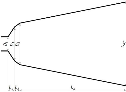
Fig. 1. Multiflare horn antenna after [22].
