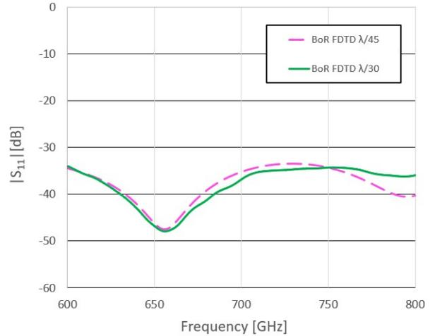
Fig. 3. Return loss,calculated by BoR FDTD at meshing of  $\lambda/30$  (CPU time 3 seconds) and  $\lambda/45$  (10 seconds).
