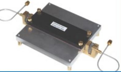
TE01δ cavities, typically 1 GHz – 10 GHz for bulk low-loss dielectrics
