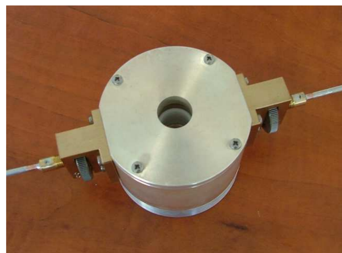
General view of TE 01δ dielectric resonator for liquid or powder sample measurements
