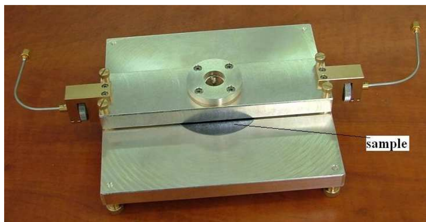
General view of single post-dielectric resonator operating at frequency about 10.8 GHz
