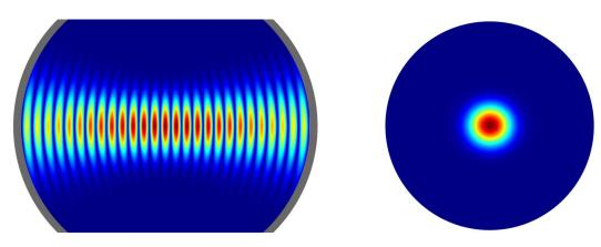
Odd  $\text{TEM}_{0,0,q}$  **Gaussian modes**, where *q* is a longitudinal mode order, are exploited in the extraction of the complex permittivity of a dielectric sheet inserted exactly in the middle of the cavity.
