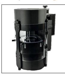
Our flagship product dedicated to accurate and robust characterization of dielectric sheets in the 15-130 GHz frequency band in just a few minutes. It provides dielectric constant and loss tangent with the inaccuracy less than 0.5%.
