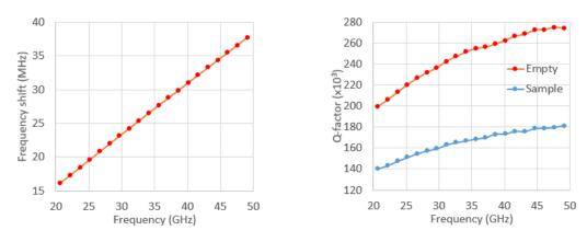
By comparing measurement results with the EM model of the FPOR, resonance frequency shift is translated into the **dielectric constant**, and Q-factor's decrease into the **loss tangent** of a material under test.
