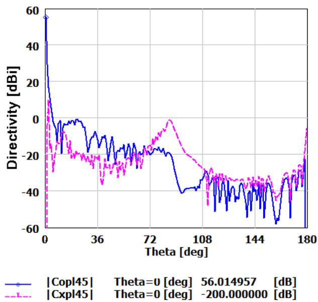
Fig. 6. Radiation pattern of the dual reflector antenna at 8.15 GHz calculated with BOR FDTD.
