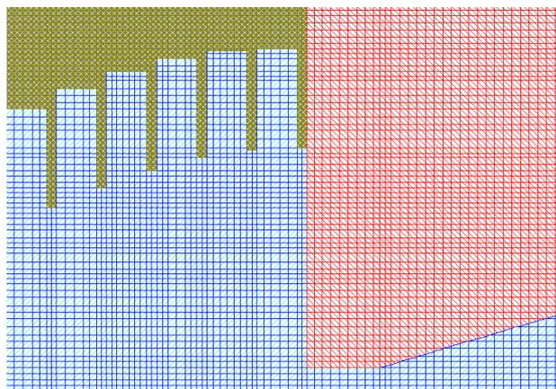
Fig. 2. An example of conformal BOR FDTD meshing as in QuickWave [4].
