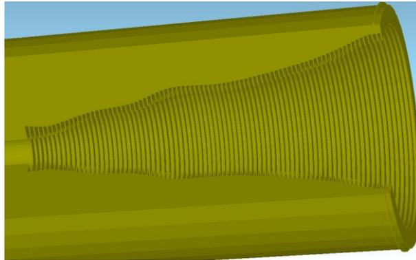
Fig. 1. An example of conformal BOR FDTD meshing as in QuickWave [4].
