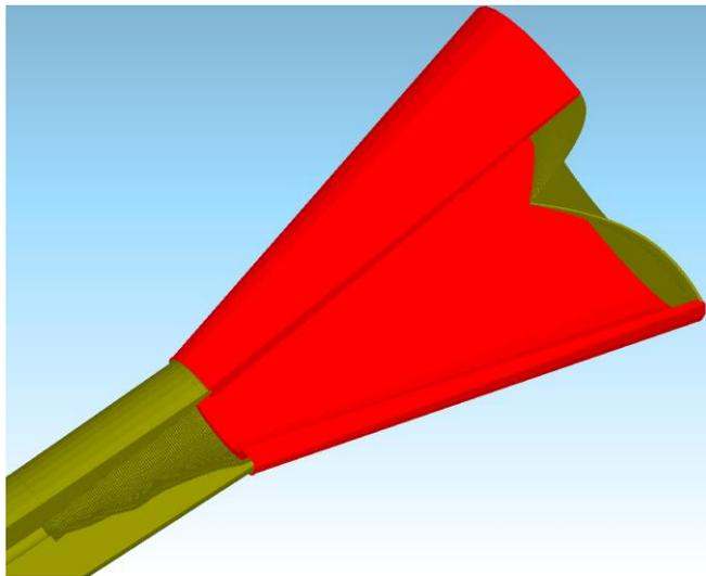
Fig. 5. Secondary reflector (subreflector) of the dual-reflector antenna system with the feeding horn and the dielectric supporting tube (low-loss, low dielectric constant, structural foam).
