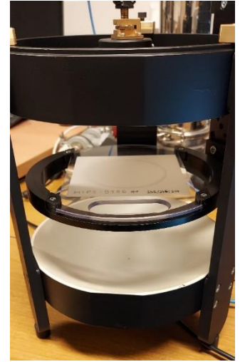
FPOR with a polystyrene (HIPS) sample placed on a sample holder
