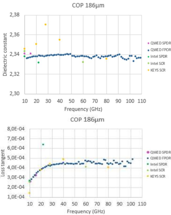
Fig. 3. Consistency of COP measurements in SCR, SPDR, and FPOR. Laboratory names in the legend denote testing sites.
