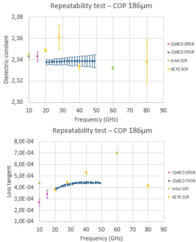
Fig. 4. Repeatability of COP measurements in SCR, SPDR, and FPOR: each symbol denotes an average of 16 measurements while error bar - triple of standard deviation. Laboratory names in the legend denote testing sites.
