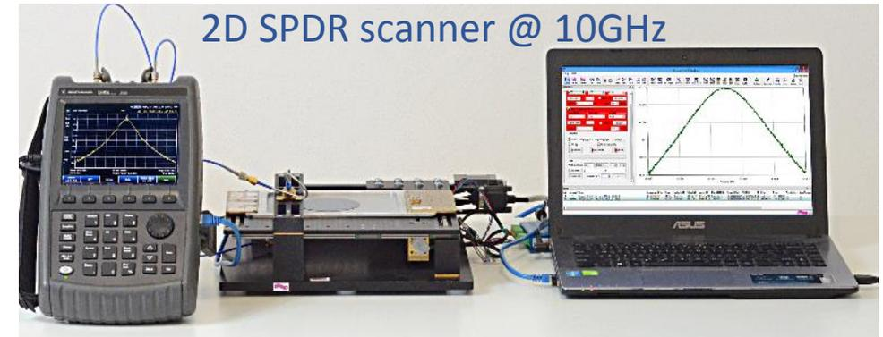
Fully automated measurement procedure through control application
