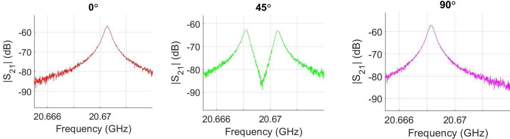
Resonances detected for **BoPET** sample ( $t = 0.100$  mm), turned in  $xy$  plane.
