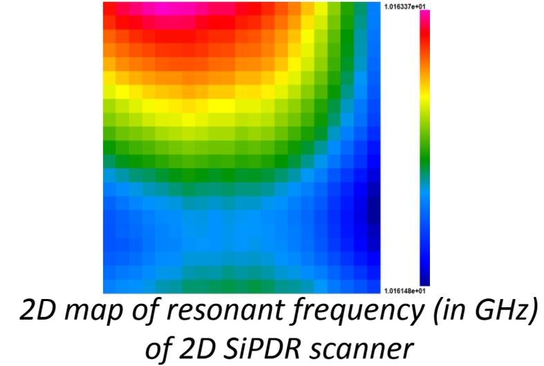
2D map of resonant frequency (in GHz) of 2D SiPDR scanner
