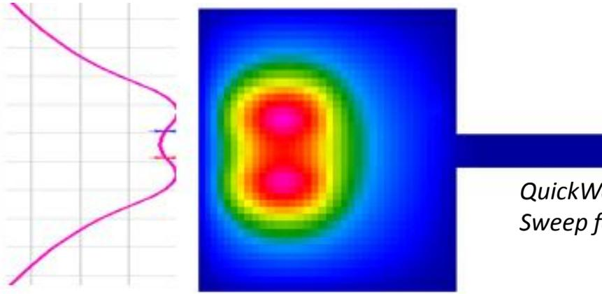
QuickWave simulations of 2.5GHz SPDR performed in automatic Parameter Sweep for varying sample thickness (colours) and dielectric constant (eps)
