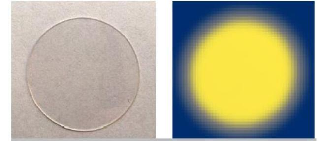
2D surface map of resistivity of semiconductor wafers
