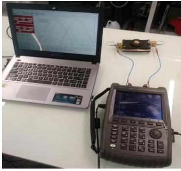
Fig. 2. Example of a portable setup applicable in the industrial environment (10 GHz SPDR, hand-held VNA, and laptop running a control application).
