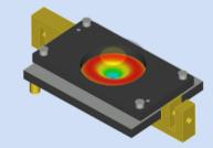
Dedicated to measurements of low-loss materials at frequencies: 1.1 1.9, 2.5, 5.1, 10 and 15 GHz
