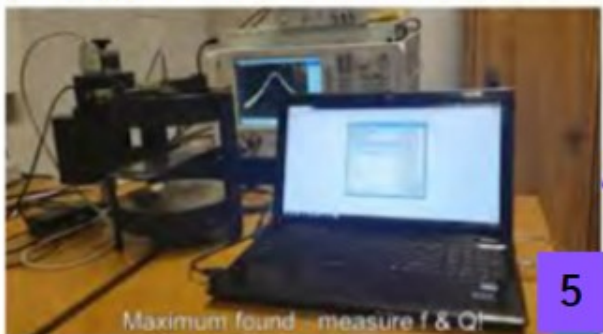
5. Material parameters at consecutive frequencies (modes) are extracted automatically.
