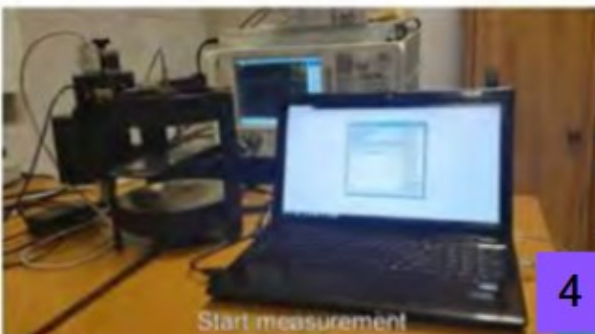
4. Automatic procedure finds M..N modes of sample-loaded FPOR.
