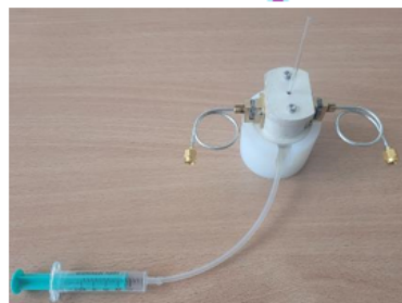
24-GHz Cavity resonator (with fused silica tube, rubber tube and syringe)
