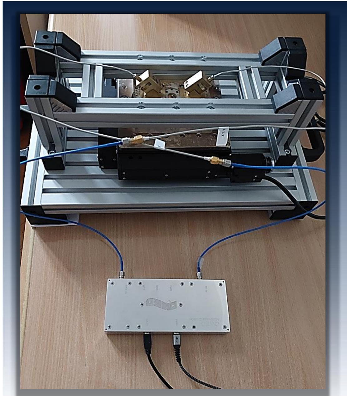
Fig. 1 Measurement setup for 2D imaging of Graphene-Based Polymer Composites: 2D iSiPDR 10GHz scanner and dedicated Q-Meter
