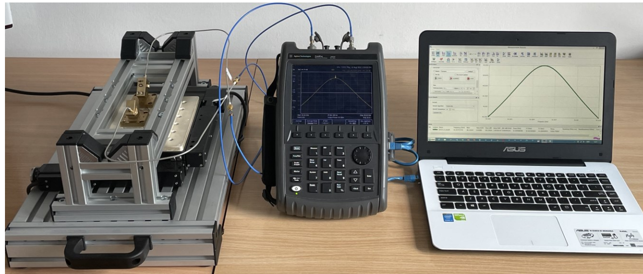
2D iSiPDR scanner based on inverted 10 GHz SiPDR
