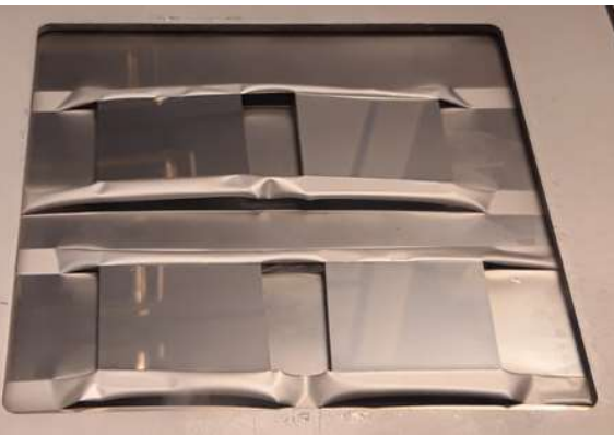
Li film on 5x5 cm 2 glass (left) and 10x10 cm 2 Cu substrates
