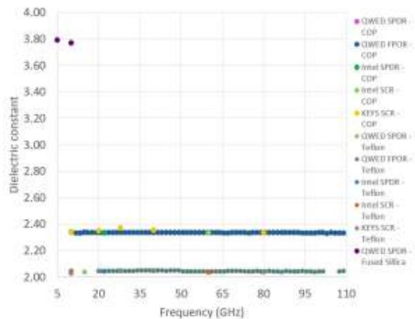
Fig.2. Summary of results of dielectric constant measurements obtained by SPDR, SCR and FPOR methods for Cyclo Olefin Polymer (COP), Teflon and Fused Sillica.
