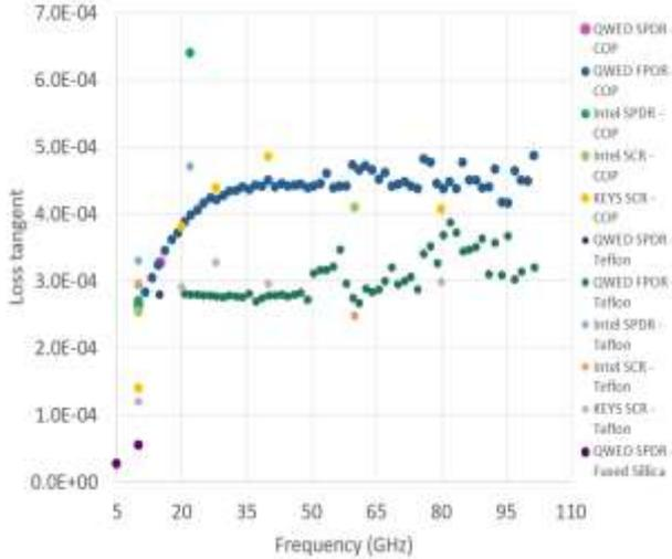
Fig. 3. Summary of results of loss tangent measurements obtained by SPDR, SCR and FPOR for COP, Teflon and Fused Silica.
