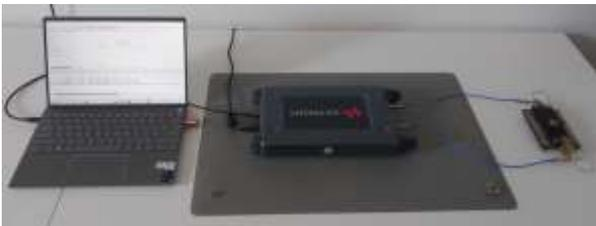
Fig.1. SPDR measuring station using VNA Keysight P5008 Streamline and dedicated software.
