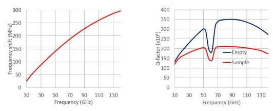
By comparing measurement results with the EM model of the FPOR, resonance frequency shift is translated into the **dielectric constant** (Dk) and Q-factor's decrease into the **loss tangent** (also known as dissipation factor, Df) of a material under test.
