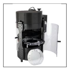
Our new product dedicated to automated broadband and accurate measurements of dielectric properties of low-loss liquids in 15 – 50 GHz frequency range. It provides dielectric constant and loss tangent with the inaccuracy less than 1%.
