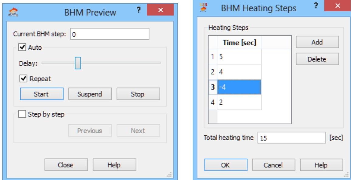
The *BHM Heating Steps* dialogue can be invoked from *Heating Details* dialogue and it allows defining different heating time for each BHM step.
