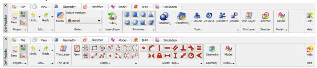
*Model* ribbon enables configuring the circuit parameters, adding ports and setting excitation, defining boundary conditions, mesh settings, and simulation parameters for *QuickWave* electromagnetic simulator.
