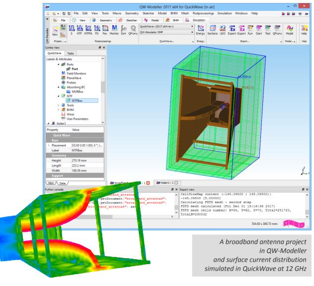
The Ribbon of *QW-Modeller* groups all necessary menus and commands that guide the user during project preparation, setting of the simulation parameters, and simulation starting process.
