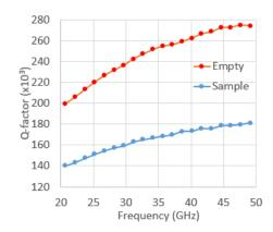
By comparing measurement results with the EM model of the FPOR, resonance frequency shift is translated into the **dielectric constant**, and Q-factor's decrease into the **loss tangent** of a material under test.
