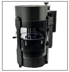
Our flagship product dedicated to accurate and robust characterization of dielectric sheets in the 15-130 GHz frequency band in just a few minutes. It provides dielectric constant and loss tangent with the inaccuracy less than 0.5%.
