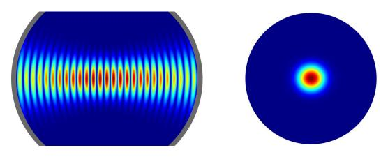
Odd  $TEM_{0,0,q}$  **Gaussian modes**, where q is a longitudinal mode order, are exploited in the extraction of the complex permittivity of a dielectric sheet inserted exactly in the middle of the cavity.
